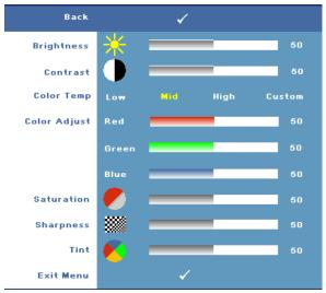
**BRIGHTNESS**—Use  $\leq$  or  $\geq$  to adjust the brightness of the image.
